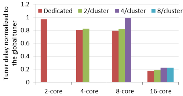
Fig. 5. Tuning delay normalized to the global cache tuner for the dedicated and clustered cache tuners ( n/\text{cluster} , where n is the cluster size) as the number of cores increases from two to sixteen cores.
