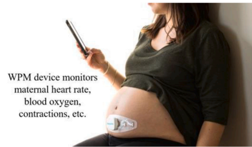
Fig. 4. Wearable pregnancy monitoring (WPM) device attached to a mother's abdomen monitors vitals of mother. WPMs require energy efficiency and high-performance necessitating application-specific hardware. Photo: Bloom-life, 2021.
